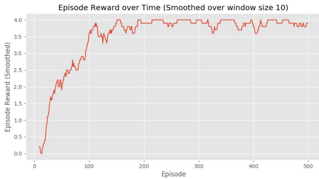
Figure 6: Convergence of Monte Carlo in a dynamic setting (each episode consists of 4 feedbacks).
